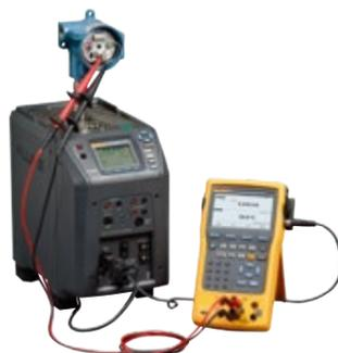
By combining the automating and documenting capabilities of the Fluke 754 Documenting Process Calibrator (see page 116) with Fluke Calibration's intelligent and stable family of field drywells and micro-baths, you have the capability to test the process sensor and the entire loop.
