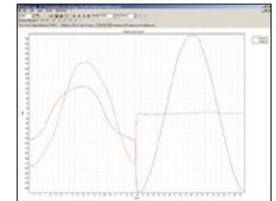
Actual transient display (> 100 μs) with time stamp – Quickly identify issues with included graphical software.
