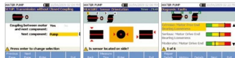
**1. Setup:** Vibration testing has never been easier. The Fluke 810 asks for basic machine information you already know, like RPM and horsepower. Its onboard info feature gives you field tips for setting up and taking measurements like a professional.
