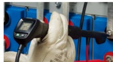
BT521 Intelligent Test Probes with integrated display
