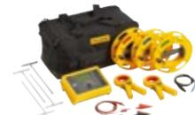
**Fluke 1623-2 GEO Earth Ground Tester Kit**
